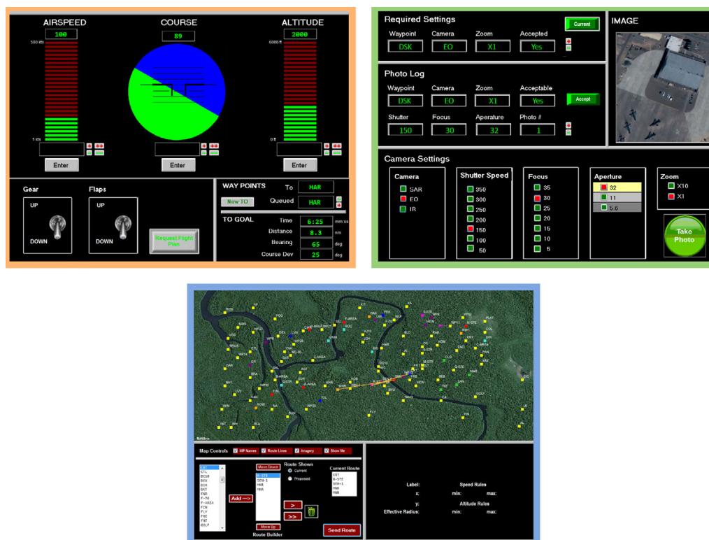
Figure 1. View of the pilot/AVO's console (Orange-Top left), view of the photographer/PLO's console (Green-Top right), and view of the navigator/DEMPC's console (Blue-Bottom).
